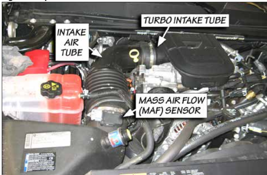
Figure 1- Separate Intake Air Tube from Stock Air Box Cover
